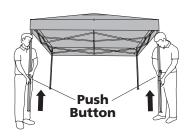
(2) Press the push buttons and release all 4 corner-sliders to collapse the frame.
